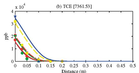
Figure 2. Sampling of large volumes of groundwater at Belgian site (left); Column feasibility test (middle); and measured and simulated TCE concentration profiles along the column (right)
