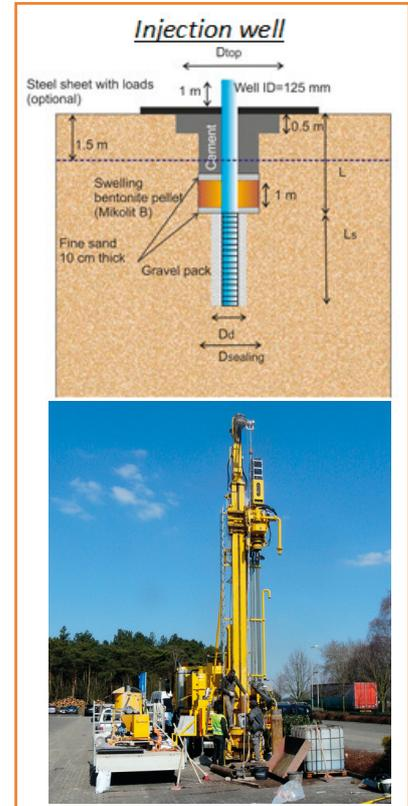
Figure 3. Design and installation of injection well
